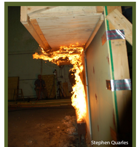
Lateral flame spread was reduced when a combustibility soffit material ignited in this test of a soffited-eave with a combustibility soffit material.
